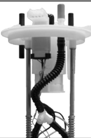
housing must be preloaded against the bottom of the fuel tank.
